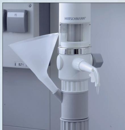
Adapter with NS 12/21 filling tube for funnel The adapter with standard ground 12/21 filling tube enables problem-free filling of medium through a funnel - without unscrewing the basic unit.
