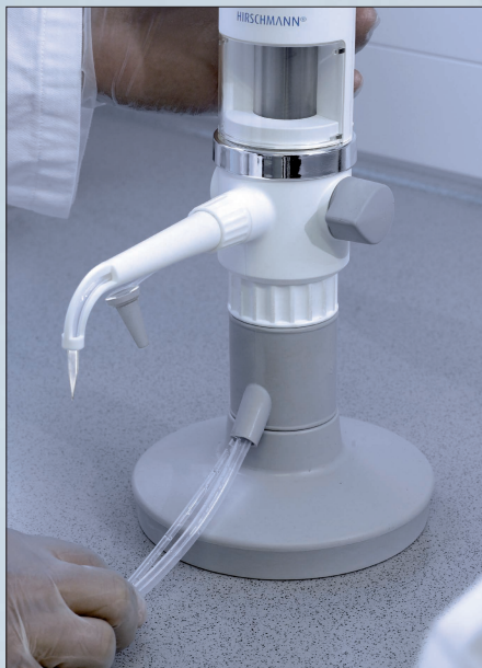
Base support instead of bottle attachment The base support enables suctioning of the medium directly from a separate storage container using a hose.
